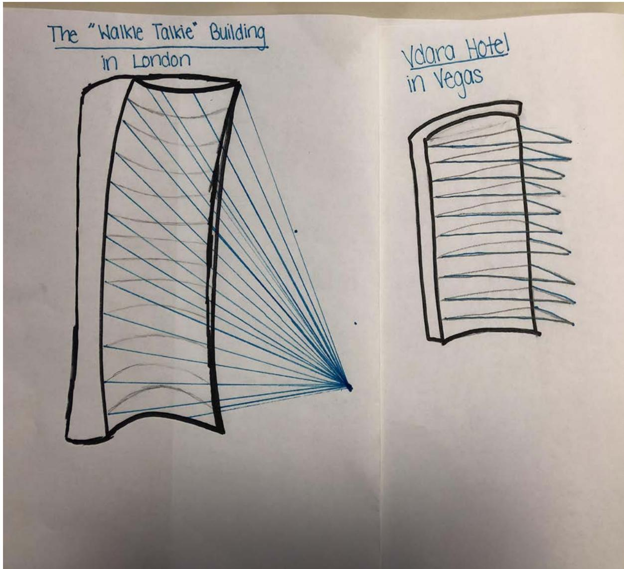
**Figure 6: This is a drawing comparing the vectors representing the reflected light rays for each building design.**
