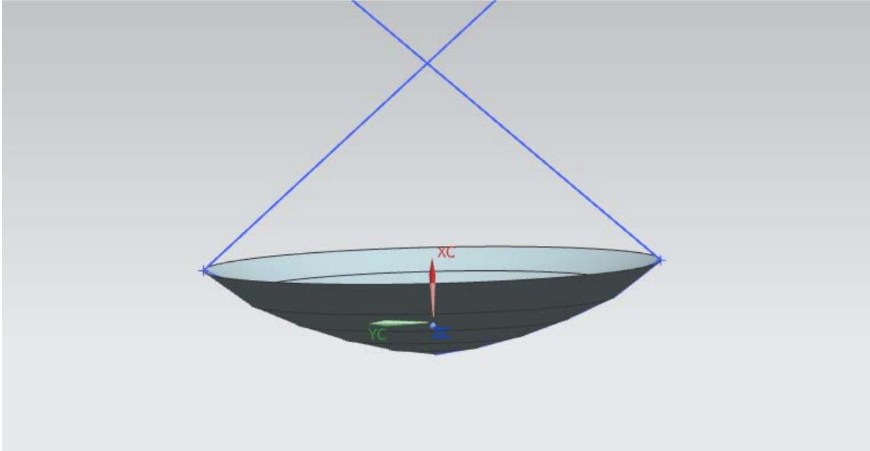
**Figure 7: This is a graphic of a negative paraboloid which we used to find the equation for  $I(y)$ . The values used to model this are the same as those in Figure 5. The intersection of the blue vectors is the computed focus.**
