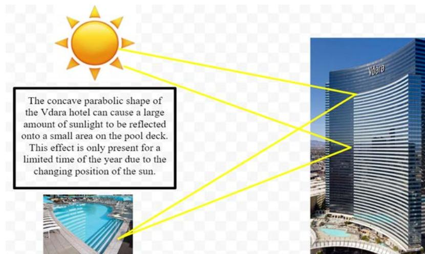
**Figure 1: This graphic, featuring the Vdara Hotel in Vegas, shows sun rays reflecting off the building toward the pool area.**
